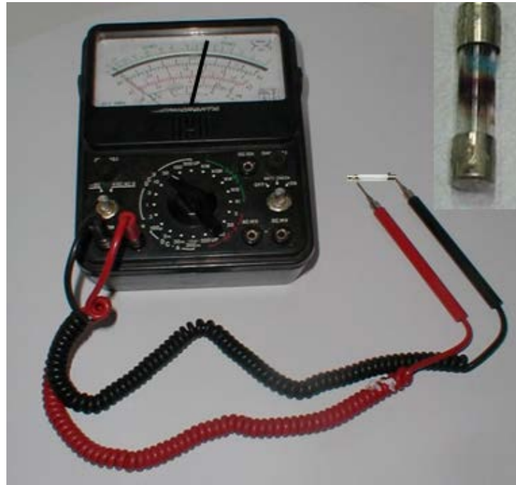
Figure 57 (from Guide & Workbook): Verifying a Fuse is Good (Shows Ohms Resistance on the Meter (left) Typical Blown Fuse (top right)
