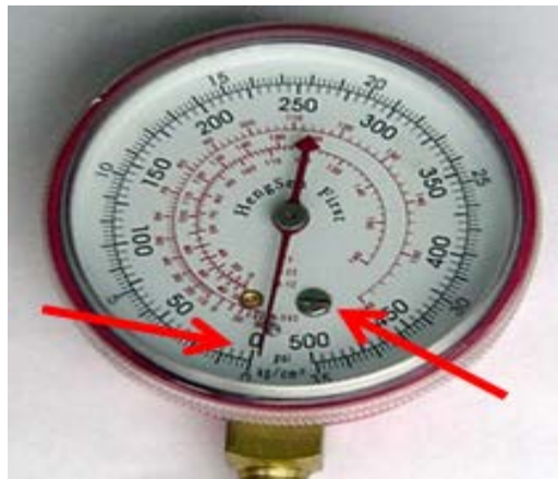
Figure 37 (from Guide & Workbook): Gauge Calibration Needle Zero Adjustment Screw
